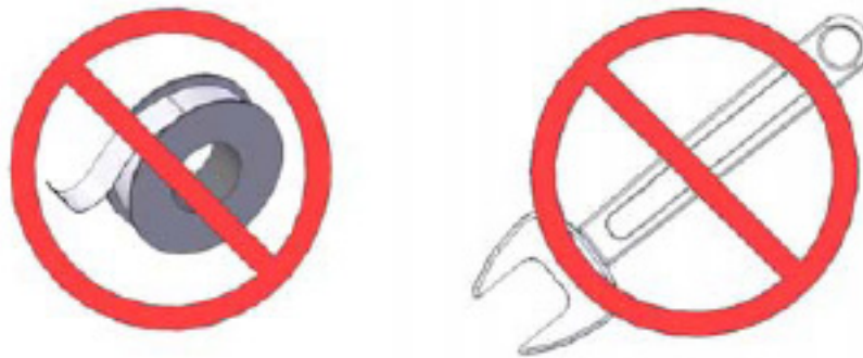
Figure 3. Hand Tighten Only
