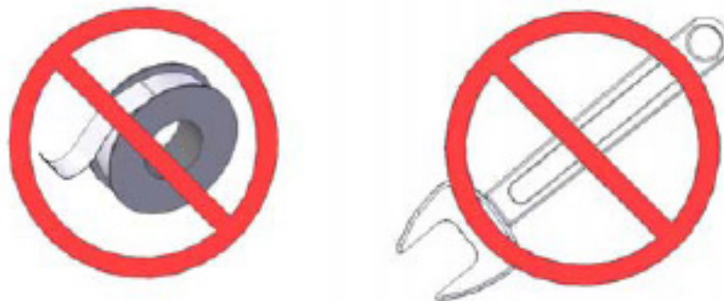
Figure 6. Hand Tighten Only
