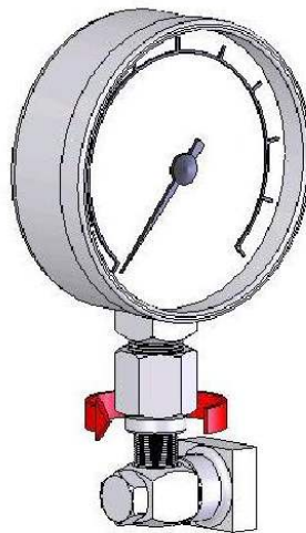
Figure 2. Connect Assembly to Test Port
