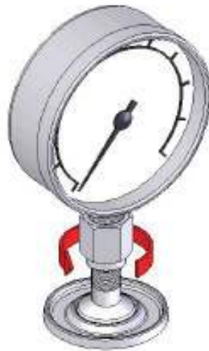
Figure 2-2. Making Pressure Connections
