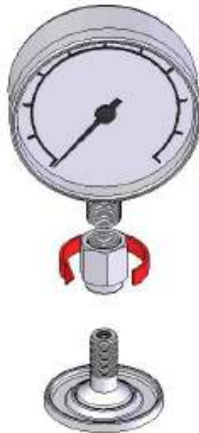
Figure 2-1. Screw on Gauge Adapter
