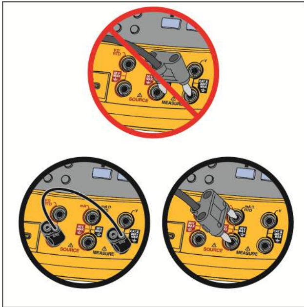
Figure 14. Correct Jumper Use
