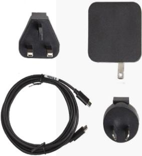
International AC Power Adapter Charger kit (includes 45 W wall charger (58 x 46 x 28 mm) with USB-C PD female port, NA plug with regional adapters (EU,UK,SAA), and a USB-C (male) to USB-C (male) cable for charging and data transfer (5 Pack). The cable can be connected to the AC adapter and TSC5 controller for charging, or from TSC5 controller to a computer for data transfer.
