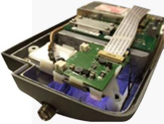
The Trimble Sentinel hardware module and application gives you real time tracking based on time or distance and allows you to easily locate lost, stolen or missing equipment. This is a service part upgrade for any S5/S7/S9/S9HP instrument and needs to be paired with the Trimble Sentinel subscription (103500-00).
