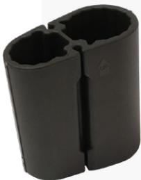
Custom-designed rubber mount for attaching a PowerCore Mini+ power bank (3350 mAH) to standard Trimble survey poles. Included in the Trimble DA1 receiver packout. Not suitable for use with the ANKER PowerCore 5000 power bank. Instead, refer to the Trimble DA2 standard accessory kit.
