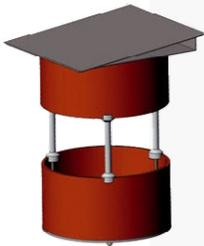
The housing is designed for use with Trimble S-series instruments. Instruments with a similar tilting axis height can be used as well. The field of sight can be extended by cutting the plastic tube. For mounting, the associated adapter is needed. The shelter is 500 mm at the highest point and 370 mm wide including the top rectangular section. The total station line of sight section in the middle is 150 mm high.
