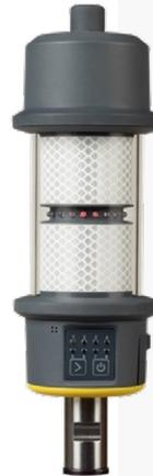
Maintain target lock with confidence using Trimble Active Tracking technology and selecting from 8 different channels. Target has 360 foil and a single ring of LEDs for Active Tracking. Includes 7.4 Li-Ion battery. Trimble standard target height 135 mm.
