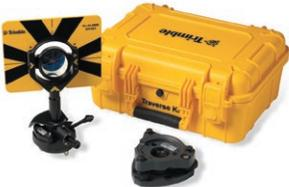
Contains case, traverse prism, prism base (with level and optical plummets) and tribrach (with no plummet). The prism base with level has a lever arm with bottom notch measurement that enables accurate height measurements and removes the need to remeasure when pairing with an S-series or SX instruments.
