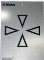
Target for checking and adjusting the alignment of the laser pointer on an S-series instrument.
