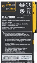
User-replaceable, rechargeable battery (8,000 mAh).
