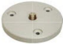
Anodized aluminium plate diameter 140 mm. The three anchor bolts embed into concrete. A 5/8" thread in the center is used for instrument mounting. A cover plate (PN 1510002-MON) to protect the pillar plate is available. The pillar plates have a groove for the instrument housing.
