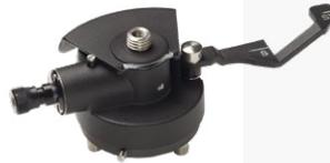
Prism base containing built in optical plummet, plate bubble for accurate leveling and lever arm for accurate height measurements to bottom notch for both S-series and SX10 total stations.
