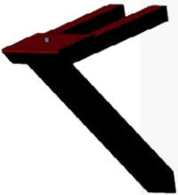
Total station mount, wall console made of robust 500 mm steel angle section. The red coating makes it well visible and corrosion-resistant. The ground plate has a 5/8" thread for instrument mounting. The console will be mounted by using the provided high power dowels, or M12 anchors can be used. As an option the 5/8" thread screw can be delivered separately. Size of the ground mounting plate is 200 x 200 x 10 mm. The steel angle section is 500 mm in length.
