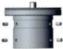
Plate with adapter for mounting on a pole. Available for different pole diameters: up to 70 mm (PN 5142120-01-MON) and up to 110 mm (PN 5142120-02-MON).
