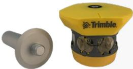
This 360 prism is compatible with all optical instruments and also supports all GNSS receivers for integrated surveying with a built-in 5/8 th thread. A levelling bubble is also included, built into the 5/8th thread. Perpendicular markings on the prism cap simplify offset measurements. Includes height adapter to Trimble standard target height (135 mm). Height adapter is used in conjunction with the telescoping rod.
