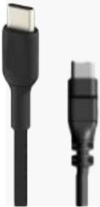
Optional 1.2 m cable for the DA1/DA2. Ends with a USB Type C connector. Provides data communications between the DA1 and Android devices. Can also be used for powering the Trimble Catalyst DA1/DA2 receiver via USB-C power-delivery equipped power banks, phones and tablets.
