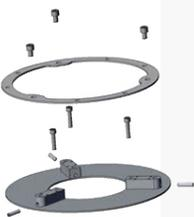
Ring with base protection plate for direct mounting at pillar plate with groove (PN 1510011-02-MON), at the pole adapter (PN 5142120-01-MON or PN 5142120-02-MON) or for mounting at the universal wall console (PN 5141250-MON). By mounting at the wall console three threads M8 have to be tapped. As an option the wall console can be ordered ready for installation of the housing. The ring is 330 mm in diameter and has a height of 35 mm.
