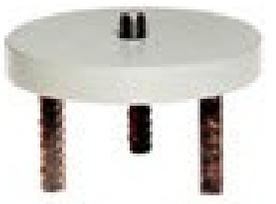
Anodized aluminium plate, diameter 140 mm. The three anchor bolts embed into concrete. A 5/8" thread in the center is used for instrument mounting. A cover plate (PN 1510002-MON) to protect the pillar plate is available. The pillar plates have a groove for the instrument housing.
