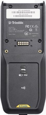
A “sled” that takes the Empower concept further to allow an EM120 Cirronet radio module to support not only Trimble Empower host devices (e.g. Trimble TSC7 controller) but also on non-Empower enabled devices.
