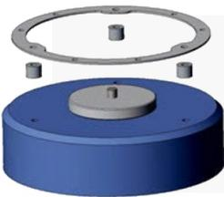
Ring including three spacers for screw mounting on top of a concrete pillar. The pillar diameter has to be larger than 350 mm.
