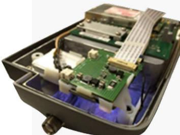
The Trimble Sentinel hardware module and application gives you real time tracking based on time or distance and allows you to easily locate lost, stolen or missing equipment. This is a service part upgrade for any S3/S6/S8/VX instrument and needs to be paired with the Trimble Sentinel subscription (103500-00).
